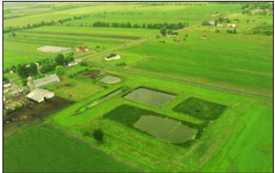
This wetland area near Embrun was constructed in the mid-1990s to treat liquid milk house wash water waste and run-off from the solid manure pile and cattle exercise yard on the adjacent dairy farm.
